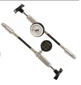
When the stress exceeds the adhesion of the coating, the dolly and coating detach from the substrate. The maximum value of hydraulic pressure during the test is recorded and is equivalent to the adhesion of the coating to the substrate.
